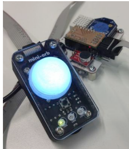
Figure 2: MiniOrb interaction device (foreground) connected to sensor device (background)
