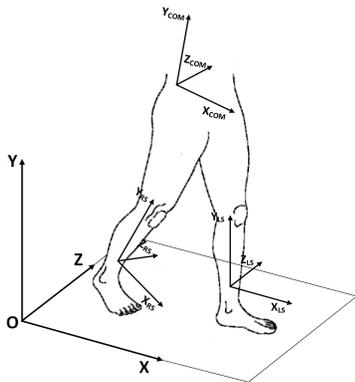
**Figure 3.** Three IMU sensors were placed on the body. One sensor on the center of mass (COM) and one sensor on each shank (LS and RS).
