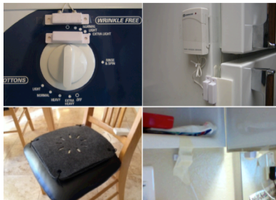
Figure 1. Exemplar use of magnetic sensors for detecting user's object use.
