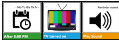
Figure 2. Exemplar composition (“If TV turned on after 8 PM, a sound clip played.”) of GaLLaG Strip
