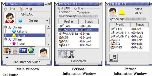
Figure 4. User interfaces of seamless agent software on multi-service user terminal (MUT).
