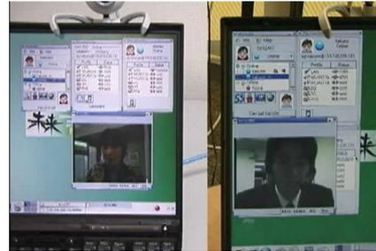
Figure 5. Laptop MUTs performing video phone through a broadband connection: left) user A's windows, right) user B's windows.
