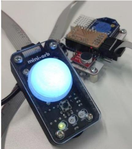
**Figure 1:** MiniOrb interaction device (foreground) and sensor device (background)
