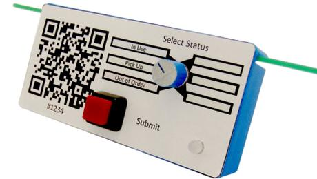
**Figure 1:** An RF-powered *Arfid* prototype controller supporting pushbutton and rotary-dial input modalities. Users scan the QR code to configure, via a web interface, the function that the tactile input controls for each individual device.
