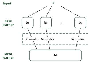
**Figure 3.** The standard score-based stacking algorithm.
